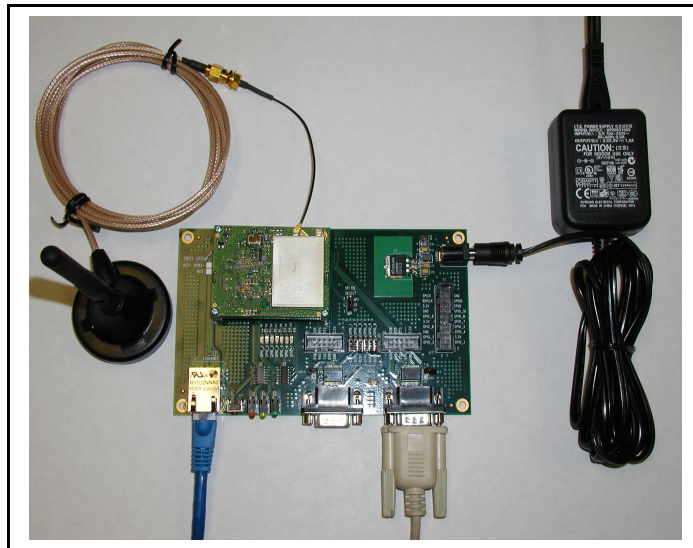
Figure 2 Installing SX-550 Module in Evaluation Daughtercard (SX-550 WLAN version shown)
